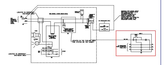
VERIFY THAT THE NEUTRALS FOR THE FIRE SYSTEM AND THE FEED TO THE MCR-1 ORIGINATE FROM THE SAME PANELS. IF NOT THEN THE COIL FROM THE MCR-1 MUST TO THE SAME NUETRAL AS THE FIRE SYSTEM
